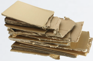
Corrugated Cardboard (wavy center layer)
